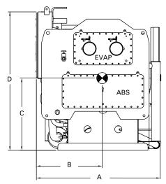
Table DW-5. Disassembly and center of gravity dimensions
